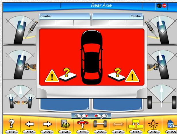
Press PAG\_UP or PAG\_DOWN keys on the keyboard to activate the automatic tracking function and launch the up or down target search.
