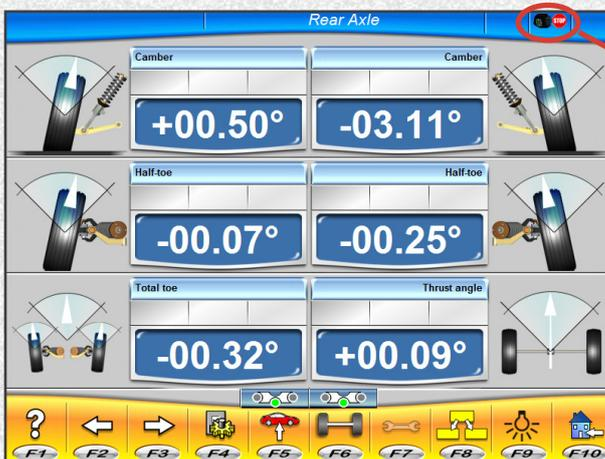
The icon highlighted shows that the automatic tracking is locked
